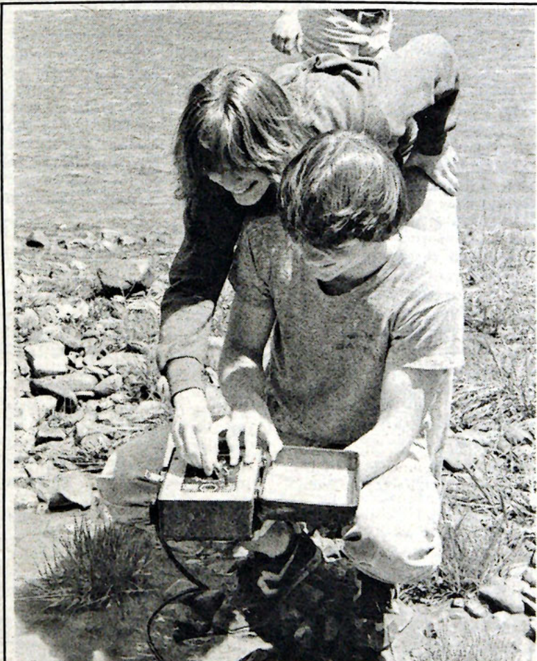
Cheryl Richardson and Brian Hill measure the specific conductance of a stream affected by acid mine drainage. Electrical conductance of water is directly related to the amount of dissolved solids in the water and is often used by water chemists during pollution assessments.
