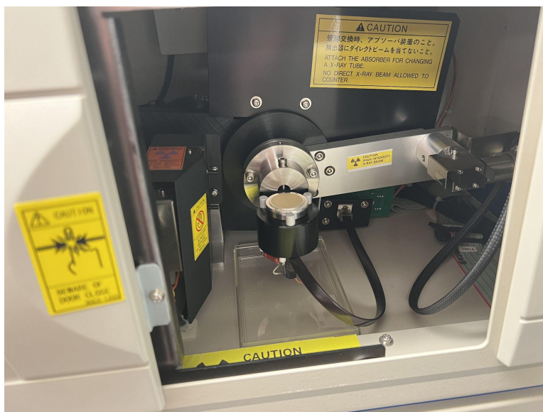
Figure 10.3. Sample bay and X-ray control arm of Rigaku MiniFlex XRD.
