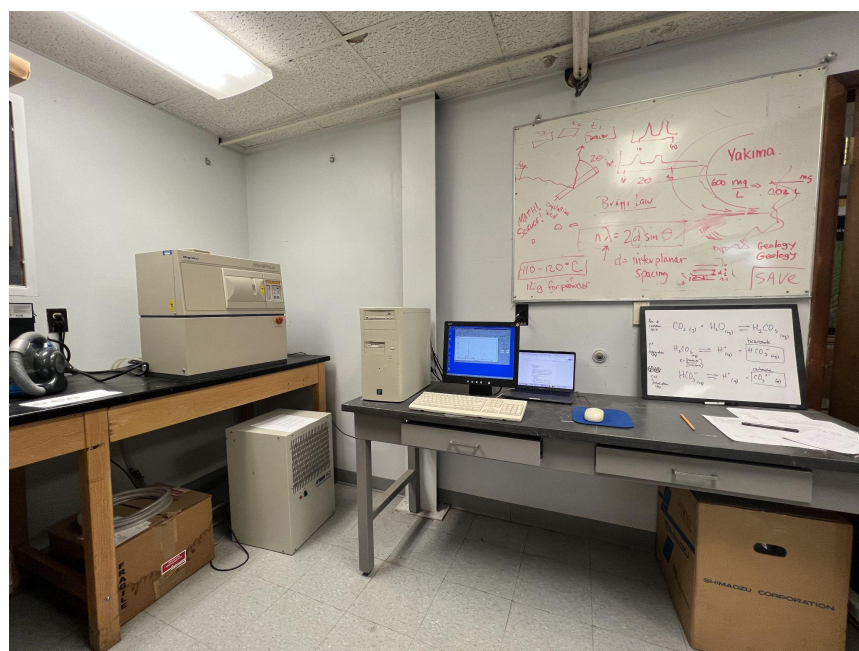
Figure 10.4. Rigaku MiniFlex XRD with attached cooling system (below XRD) and the associated computer with the necessary software for data acquisition and analysis.
